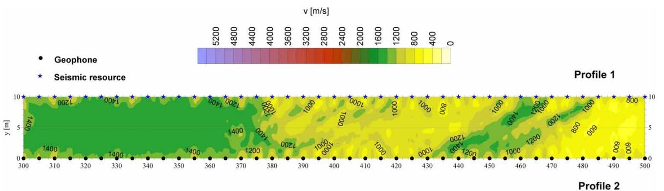
**Fig. 5** An example of result of seismic tomography between two longitudinal profiles. The measured segment is located in a place without embankment, in a cut. The locality of Montmélián
