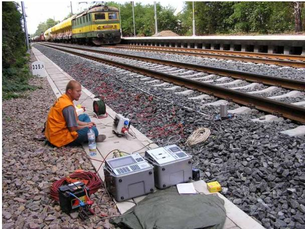
**Fig. 1** Seismic equipment McSeis 1600 OYO with seismic vibrator in the field
