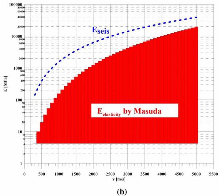
**Fig. 7** (a) The relation between deformation of a rock and modulus of elasticity  $E$  of a rock. (b) Conversion of the magnitude of longitudinal seismic velocities to the modulus of elasticity  $E_{seis}$ . This is followed by correction according to the Masuda formula
