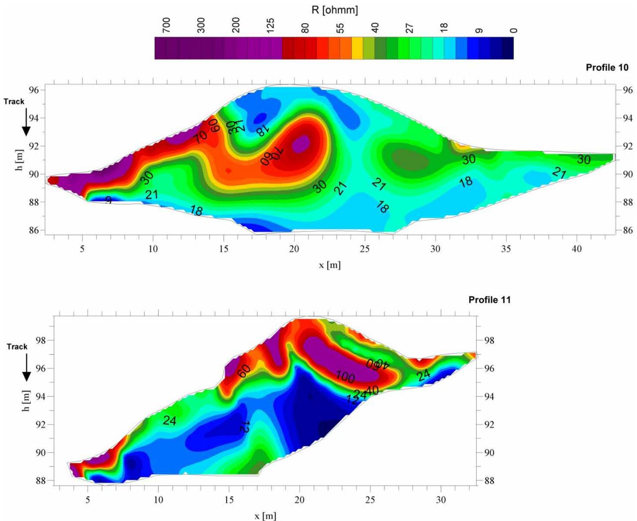
**Fig. 3** Resistivity cross-sections from the profiles running transversely to the railway embankment. The locality of Lleida
