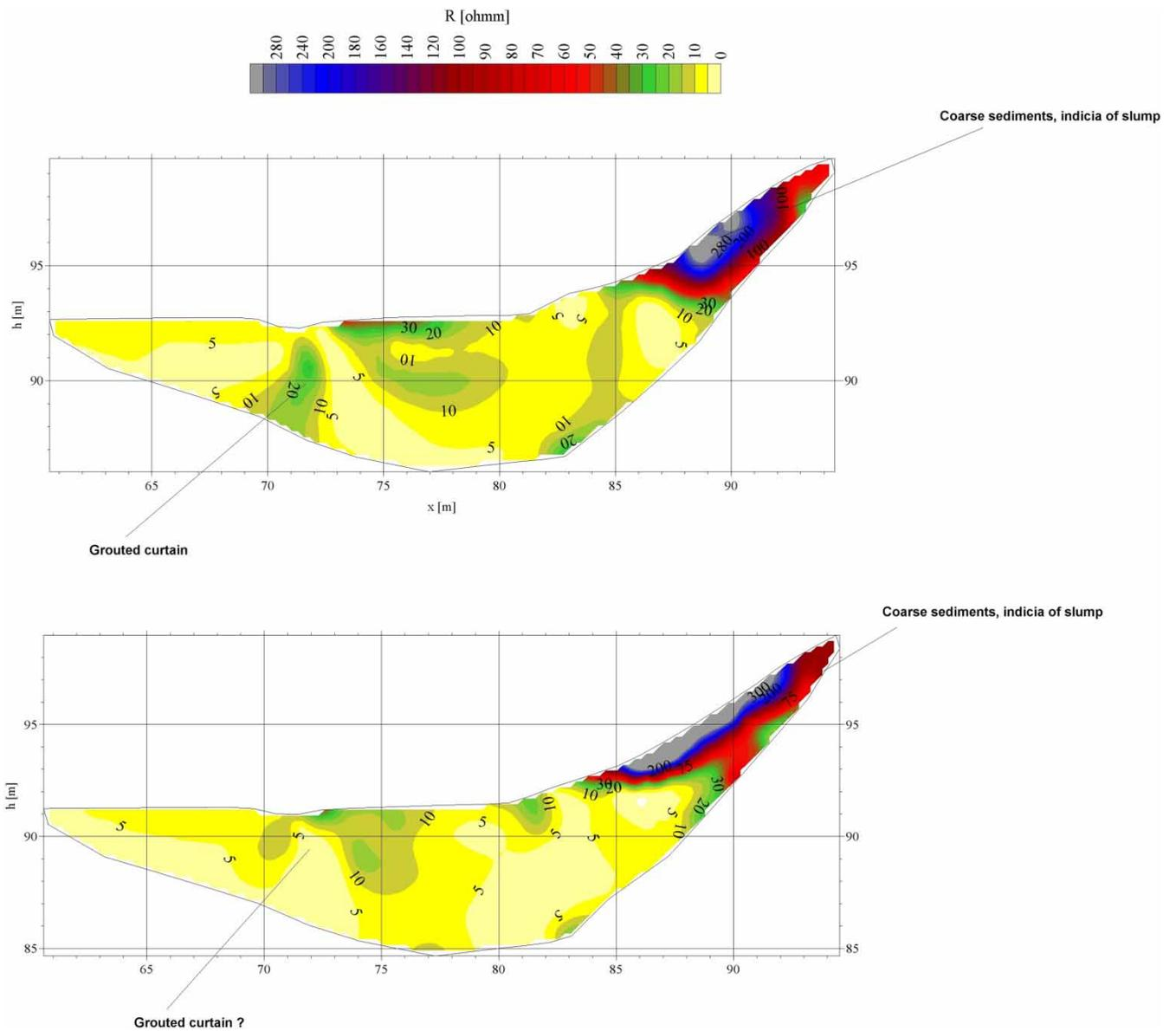
**Fig. 4** Resistivity cross-sections from the profiles running transversely to the railway embankment. The locality of Lipnik nad Bečov
