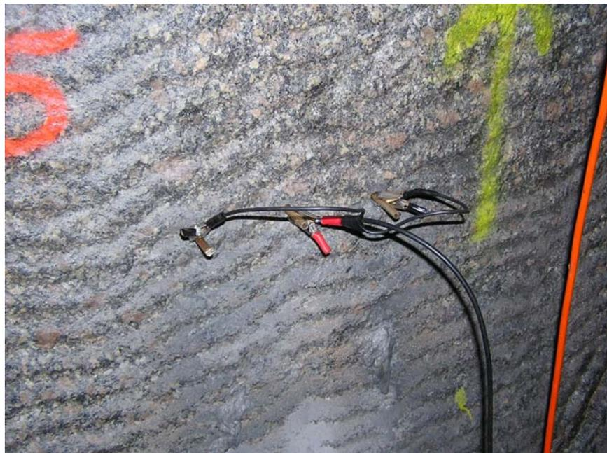
Fig. 8: Connection of electrodes for TDR measurement.
