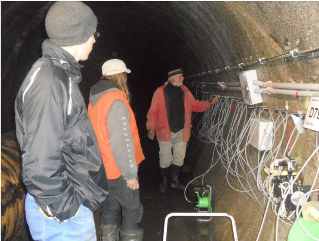
**Figure 1:** Field base in Bedřichov tunnel, metre 792. ERT system layout across the geological disturbance.
