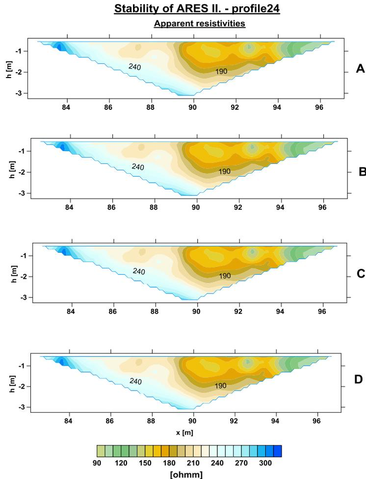
**Figure 2:** Resistivity cross sections measured at four hourly intervals at the location of Svor. Y-axis is the depth in metres (approximated by the value  $AB/5$ ).
